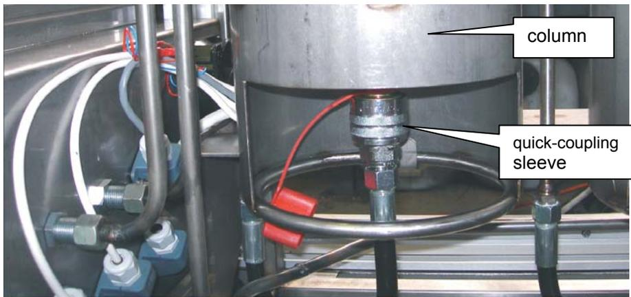
Disconnection procedure is very simple: turn sleeve in anticlockwise till decoupling
