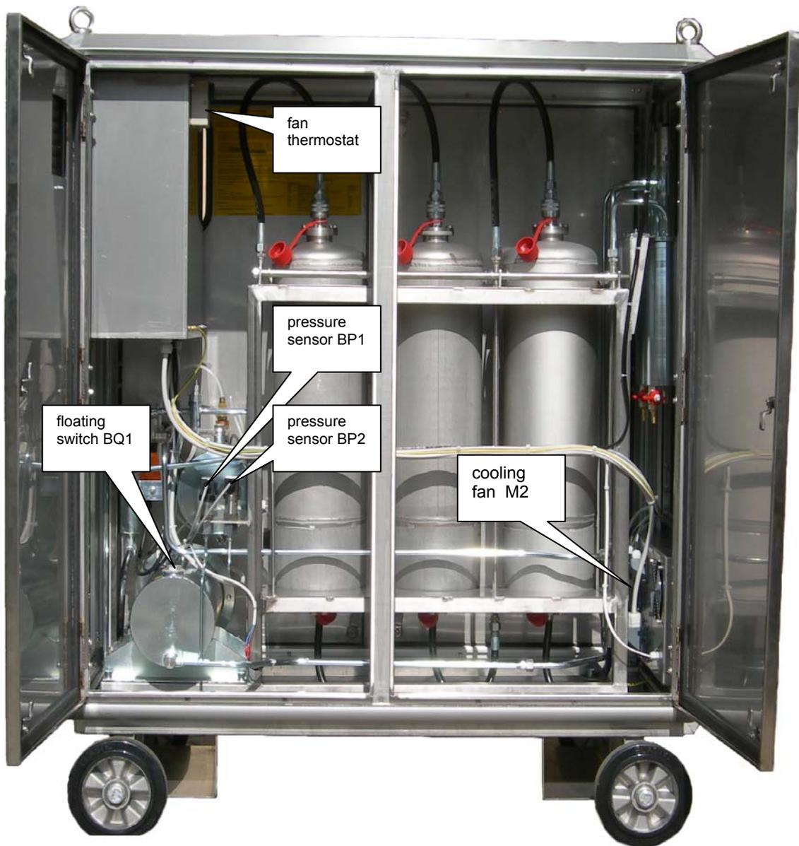
**Fig. 4** Layout of components on the back side of ADT dehydrator
