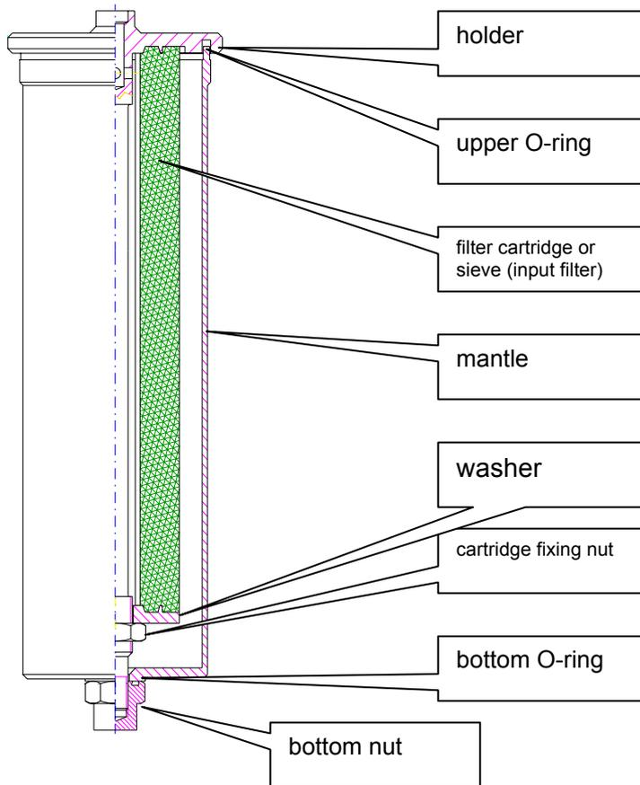
Fig. 9 Lay-out of the input and output filter
