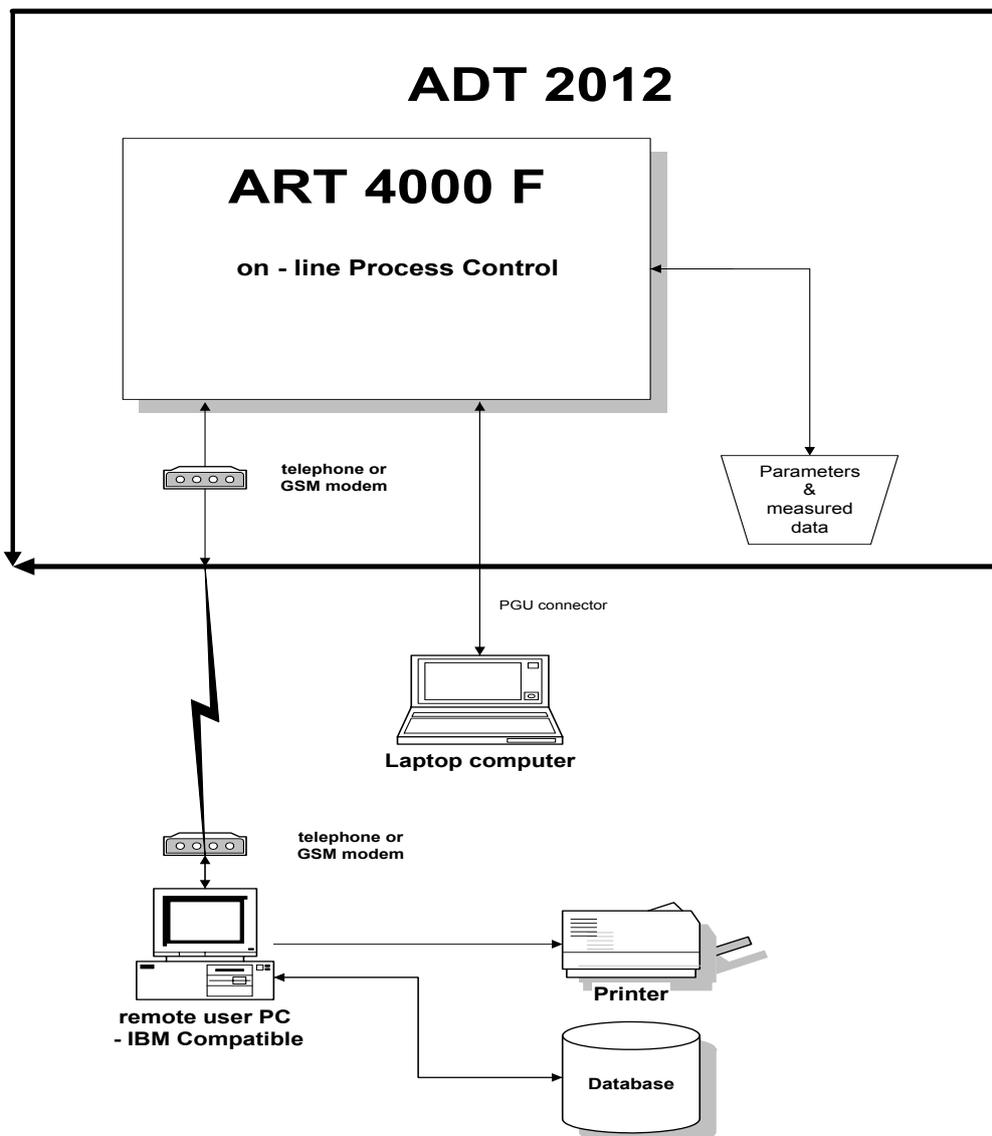
Fig. 6 Structure of control & communication of ADT
