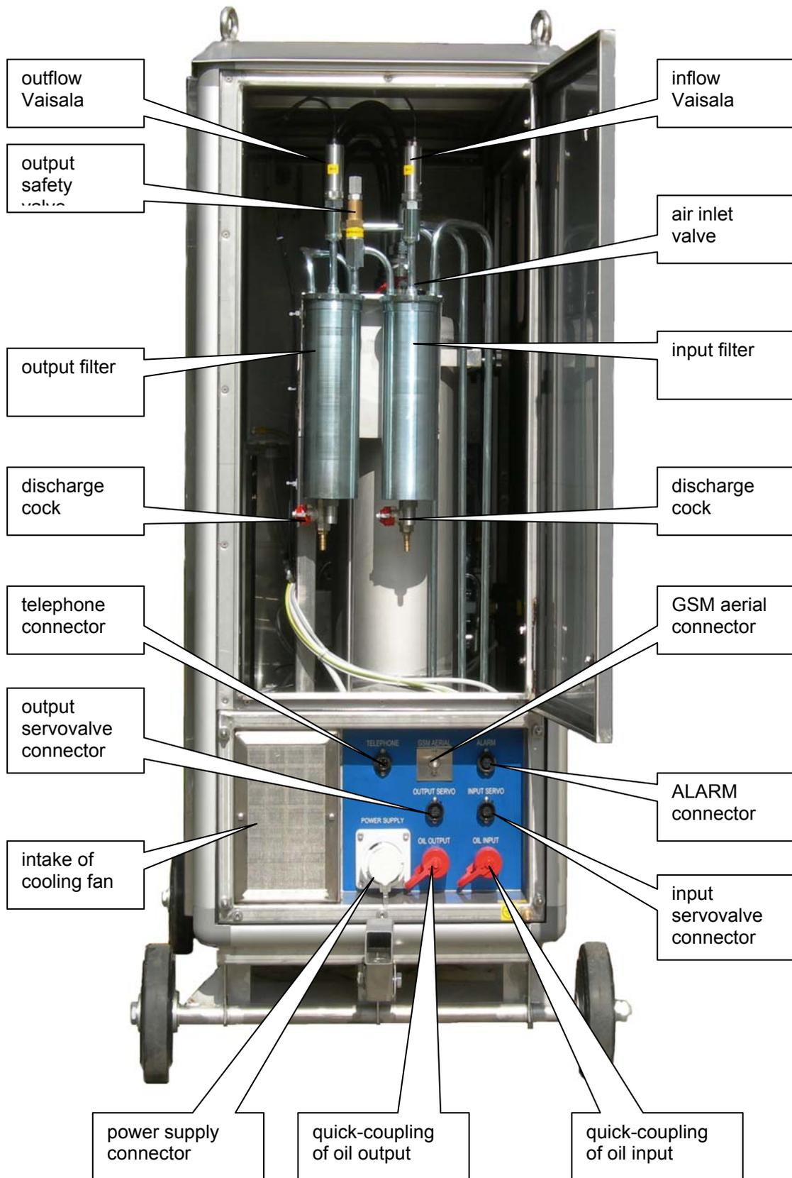
**Fig 5. Layout of main components on the left side of ADT dehydrator**
